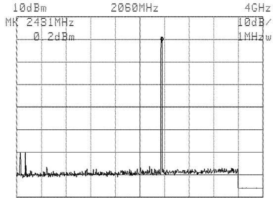
After the phone was plugged in, the radiation level rose to 673,000  $\mu\text{W}/\text{m}^2$  (+0.2 dBm) in a normally encountered distance (about 1 - 2 feet) if the base station is placed on an office desk. See figure 2. The following power density levels were obtained :
